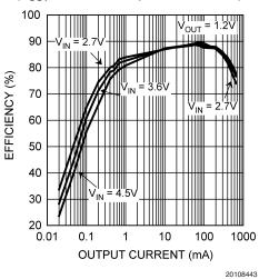
Efficiency vs. Output Current (V<sub>OUT</sub> = 1.8V, L= 2.2  $\mu$ H, dcr = 200m $\Omega$ )
