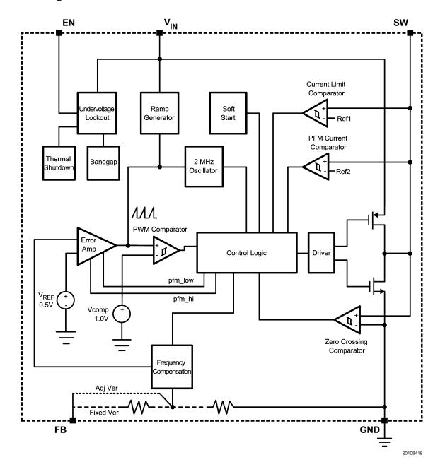
FIGURE 5. Simplified Functional Diagram
