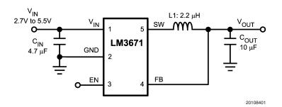
**FIGURE 1. Typical Application Circuit**
