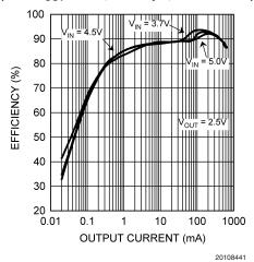
Efficiency vs. Output Current (V<sub>OUT</sub> = 1.2V, L= 2.2  $\mu$ H, dcr = 200m $\Omega$ )
