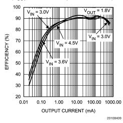
Efficiency vs. Output Current (ADJ:  $V_{OUT}$  = 3.3V, L= 2.2  $\mu$ H, dcr = 200m $\Omega$ )
