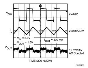
FIGURE 6. Typical PWM Operation
