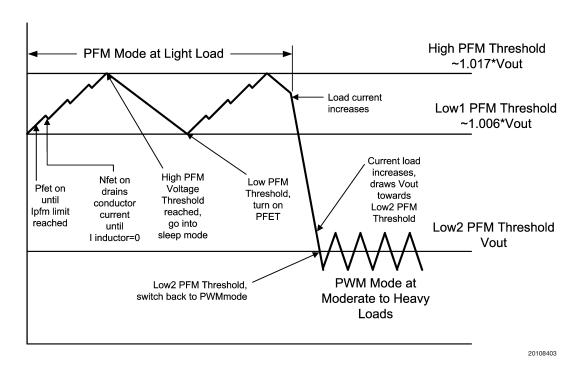
FIGURE 8. Operation in PFM Mode and Transfer to PWM Mode
